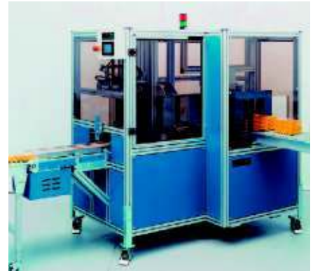
Fully automatic racking installation
