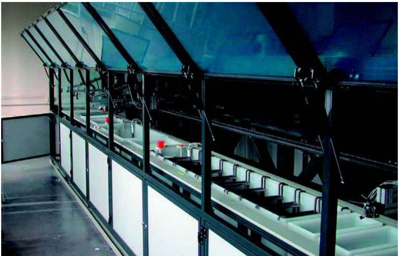
Automatic gilding plant
