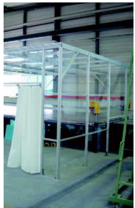
Dust protection cabin
