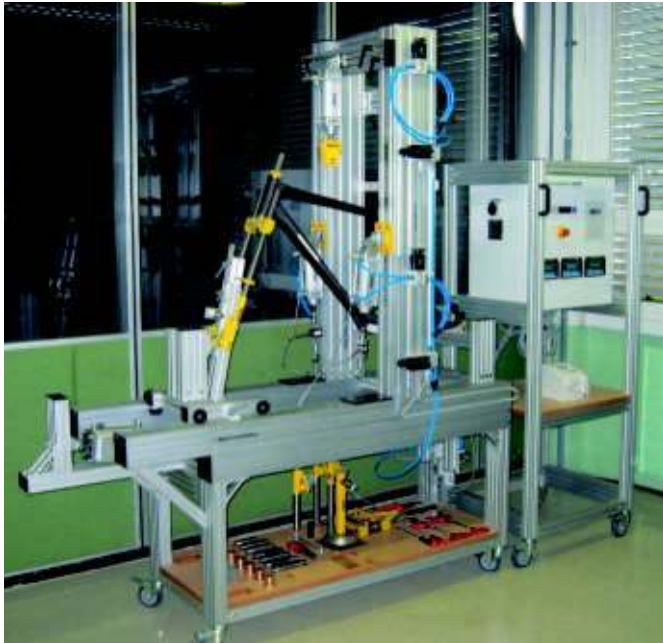
Test plant for carbonate bicycle frames
